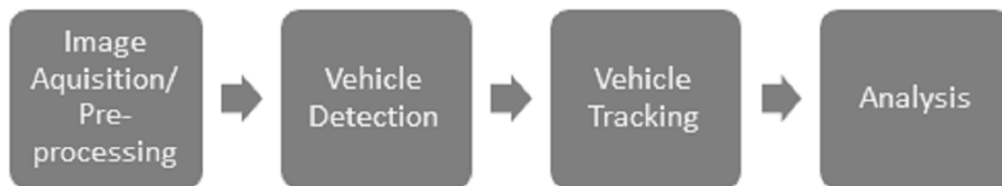
Figure 5.1. A typical vehicle detection system
