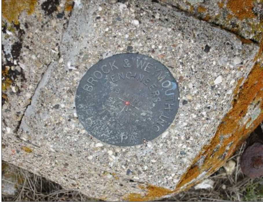
Fig. 98. National Geodetic Survey monument, designation name Williston 2 Reset, PID TG1311 Day 1. Monument is a bronze disk is mounted on top of a concrete post. USGS Quad Williston E, near Williston city dump grounds, shown also in Appendix W Benchmark #1
