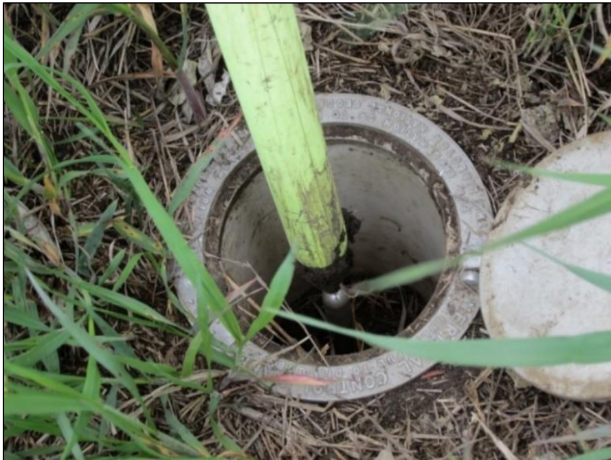
Fig. 99. National Geodetic Survey monument, designation name E 462, PID TG1543 Day 2. Monument is a covered underground 10-ft rod. USGS Quad Williston SW, near Highway-85, shown also in Appendix W, Benchmark #2
