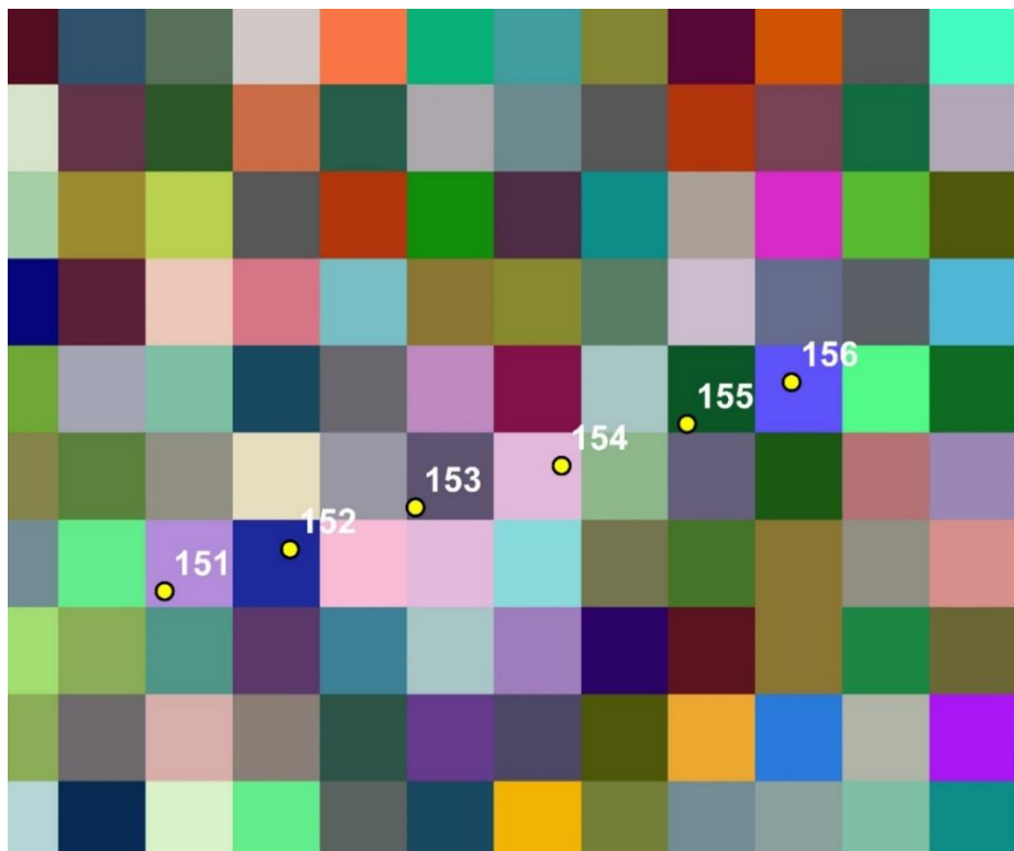
Fig. 104. Spacing of RTK-GPS control points Data sources: Intermap Technology, Inc.; KLJ Engineering; NDgisHub. Technology used: ArcInfo 10.1
