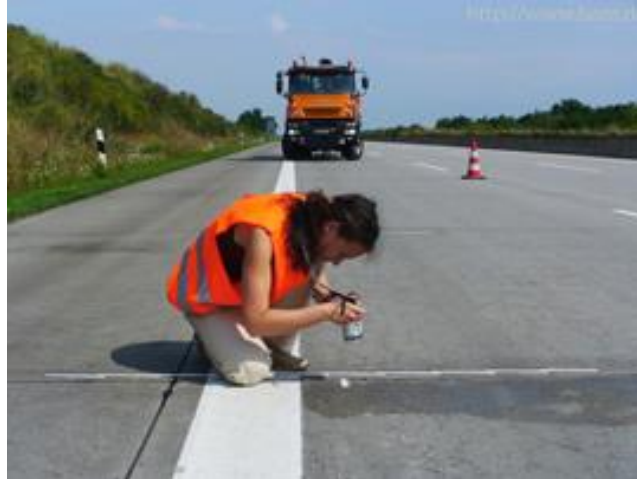
Figure 1. Manual pavement distress measurements [3].
