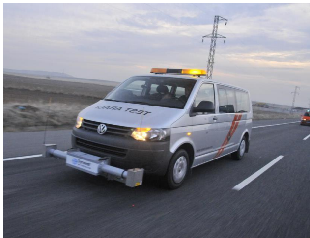
Figure 2. Standard road profiling for roughness measurements [25].
