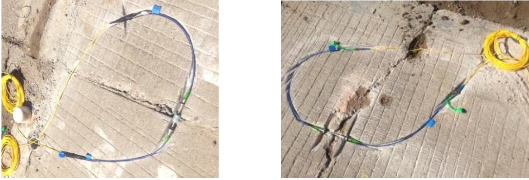
(a) Deployment of 1D-3 across the joint (b) Deployment of 1D-5 across transverse cracks
