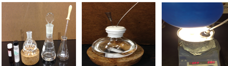
Figure 5.42: Typical photoreaction set-up for large-scale photoreaction of acrylimides.
