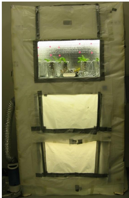
Figure 4.1. Growth chamber used for spinach study. The temperature and relative humidity was maintained at \sim 75 °F and \sim 60\% .
