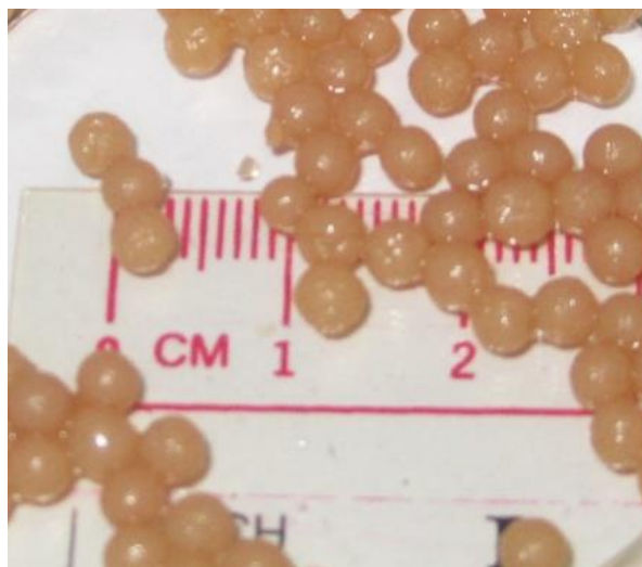
Figure 2.2. Image of the synthesized fresh Fe-cross-linked alginate (FCA) beads. The beads were approximately spherical in shape with average diameters of 3.98 \pm 0.03 mm.
