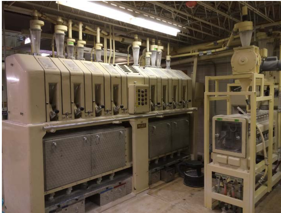
Figure 1.11. A MIAG Multomat Flour Mill Located in Harris Hall, NDSU in Fargo, ND (a) Mill Flow Diagram (b) Picture Image (Printed with permission)
