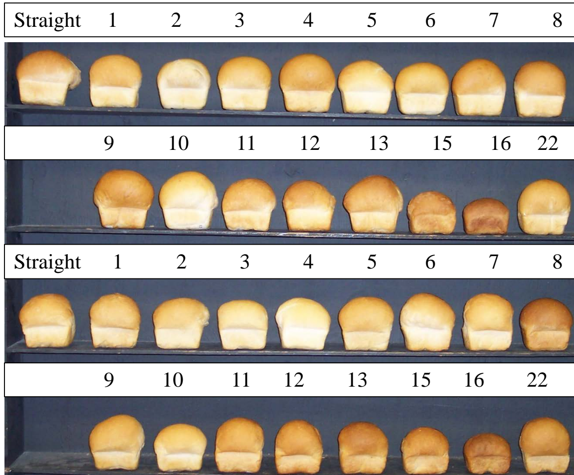
Figure 6.7. Side View Bread Pictures of Various MIAG Millstreams for ND-Glenn (top) and ND-Elgin (bottom)
