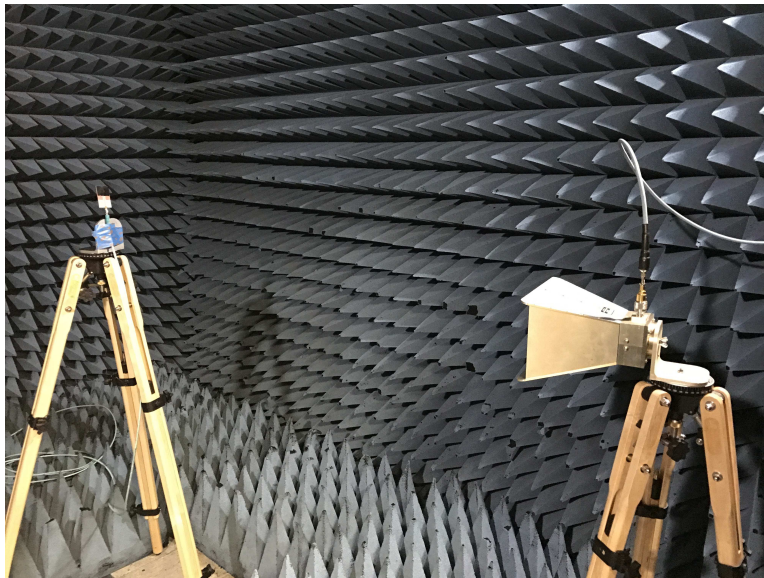
Figure 10.14. The gain measurement setup in an anechoic chamber.
