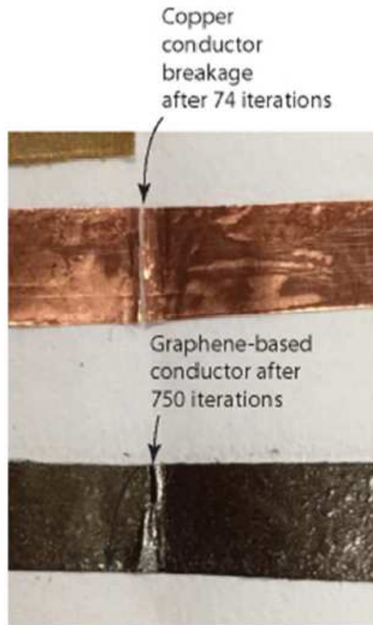
Figure 6.6. A photograph of the breakage of the copper conductor at the pivot point.
