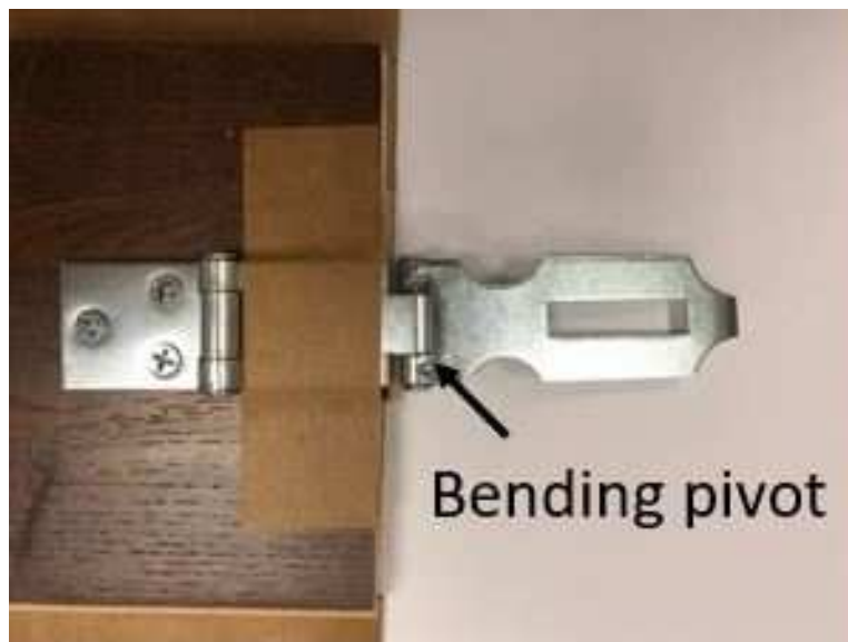
Figure 5.6. Developed test fixture for bending experiment.
