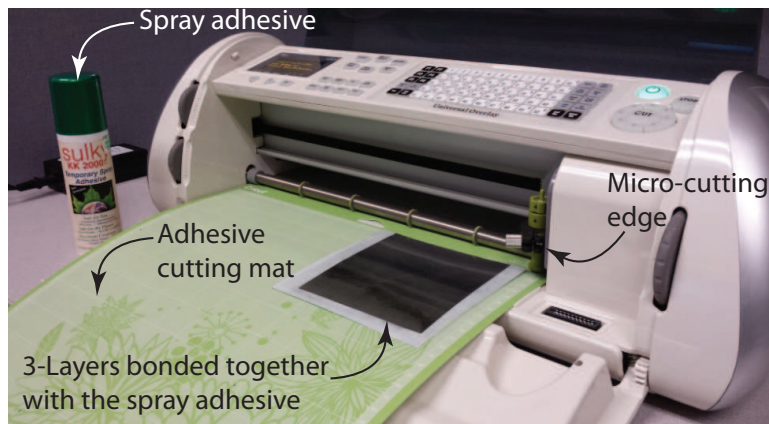
Figure 3.3. Photograph of the commercial micro-cutter [47] and the temporary adhesive spray [45].
