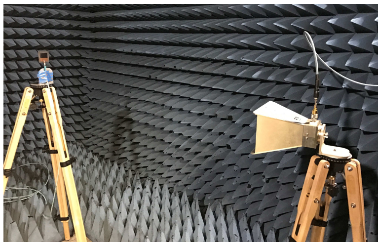
Figure 10.7. The gain measurement setup in an anechoic chamber.
