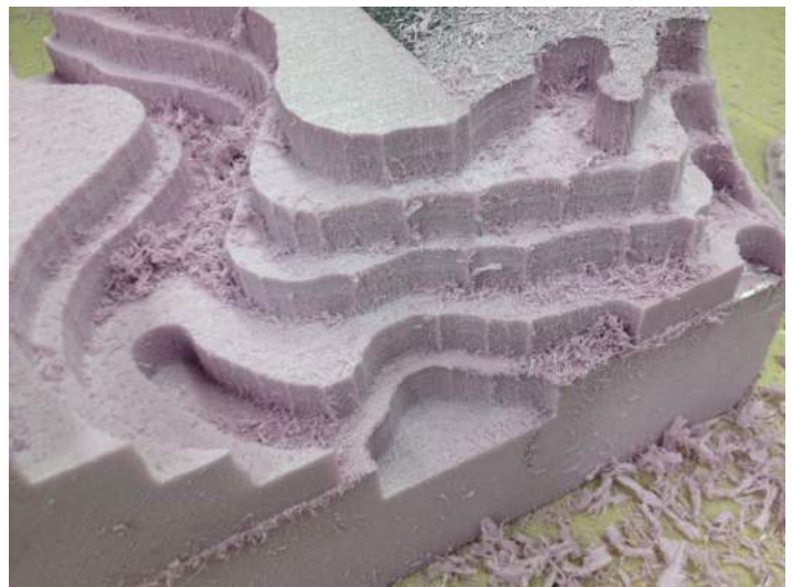
2/7 Process of Making Z Axis Models with CNC machine
