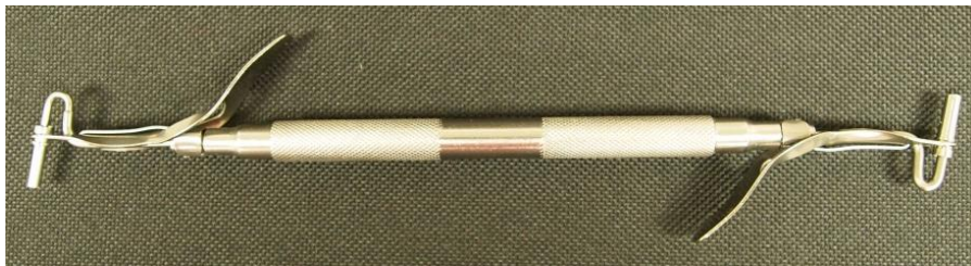
Figure 2.2. Dental amalgam tool was used to inoculate pea plants with S. sclerotiorum .
