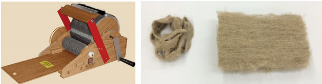
Figure 10. Carder machine used in this study and fiber before and after carding process
