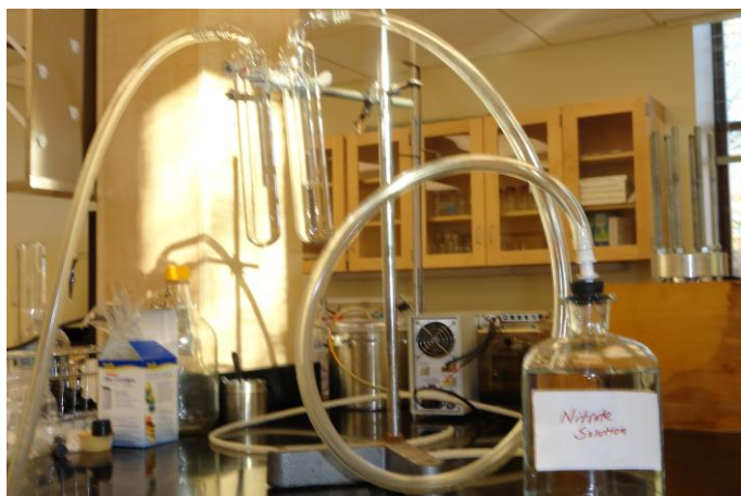
Fig 3.2 Degassing nitrate solution using Schlenk Flask.
