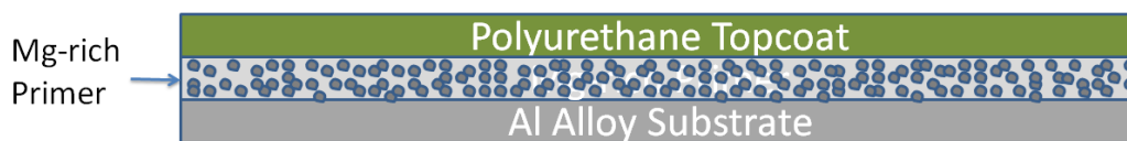
Figure 2.1. Schematic of aerospace coating systems.
