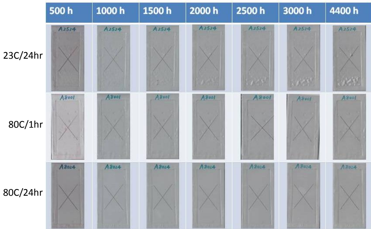
Figure 2.15. Images of scribed, topcoated Mg-rich primers derived from noTBAF system after B117 salt spray exposure as a function of exposure time and curing condition.
