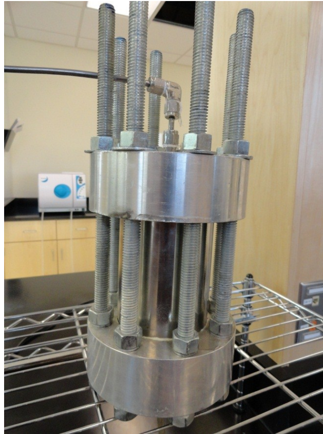
Figure 8. Photograph of the dead-end hyperfiltration cell assembly.
