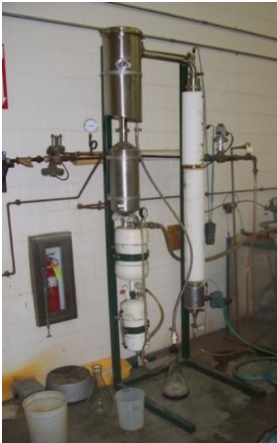
Figure C1. Rising-film evaporator used for juice concentration
