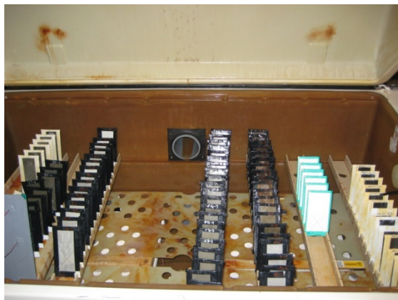
Figure 1.4: Picture of ASTM B117 salt spray chamber. [Source CPM, NDSU]
