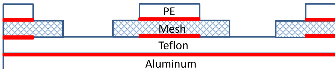
Figure 2.21. Schematic of the layers of free-film array template; the solid red colored layers represent thin adhesive layers.
