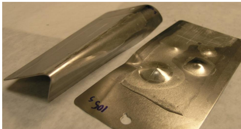
Figure 2.12. Coatings on metal panels subjected to conical mandrel bending (left) and reverse impact test (right)
