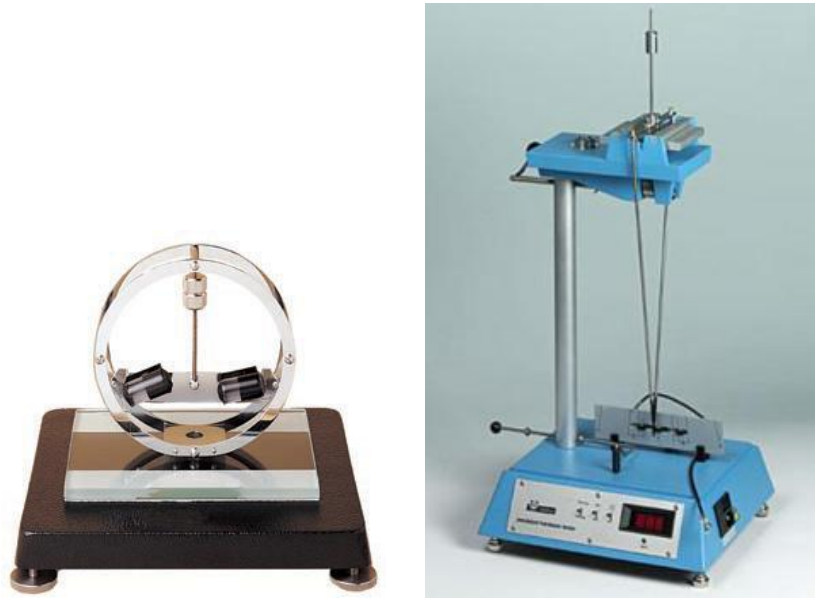
Figure 4.12. Sward type hardness rocker (left) and Konig pendulum hardness tester (right) (Reproduced from Ref. 28 )
