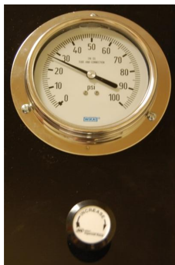
Figure 2.53. Clamping pressure gauge and control knob
