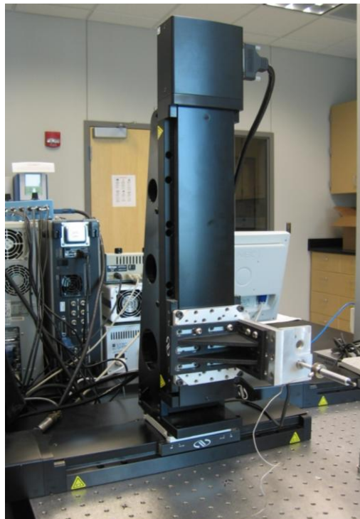
Figure 2.26. Horizontal set-up indentation
