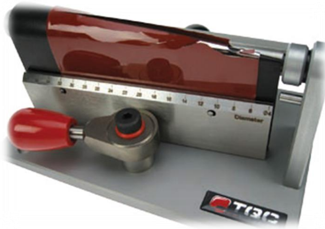
Figure 2.11. Conical mandrel bend tester (Reproduced from ref. 17 )
