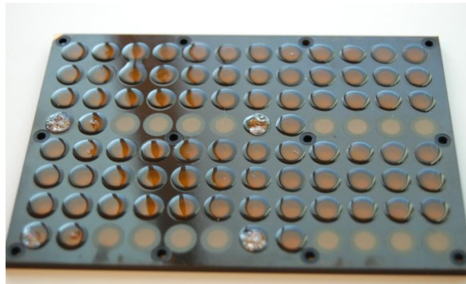
Figure 4.19. pDMTA sample plate with clear coatings
