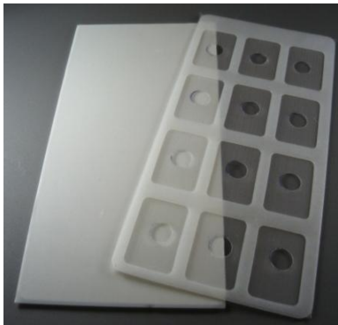
Figure 2.20. Free-film array template; Teflon substrate (left) and the circular-cut mesh on each of the 12 wells
