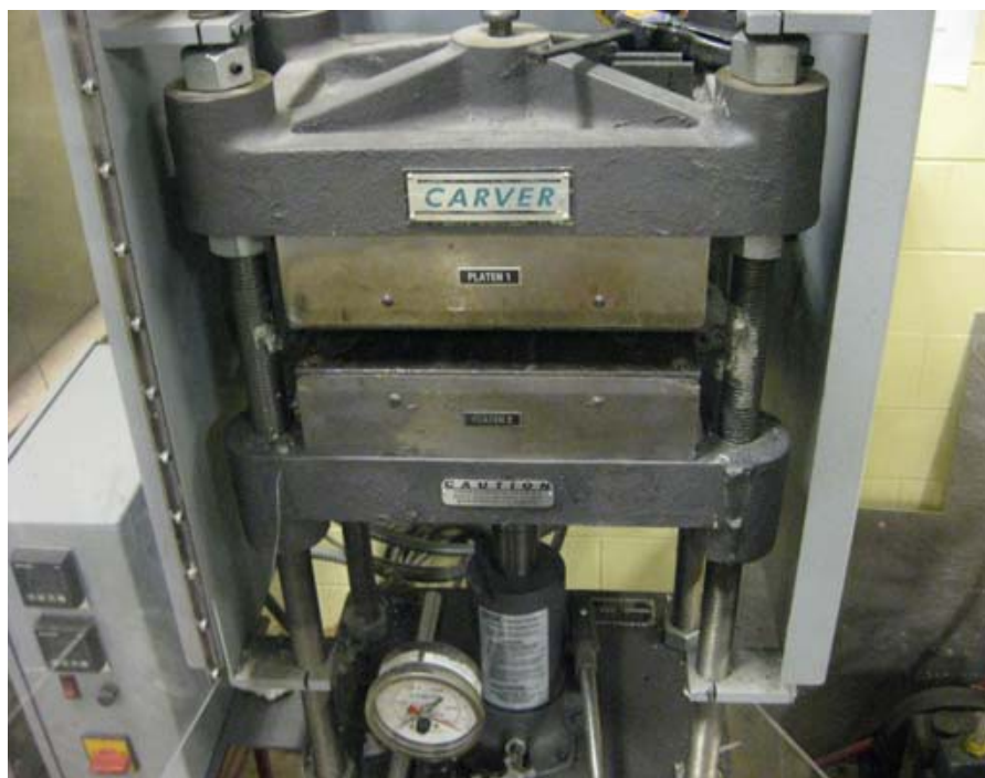
Figure 4. Carver hot press used for processing composite panels.
