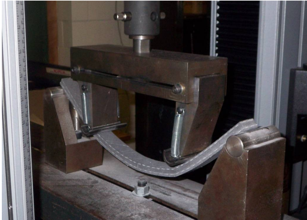
Figure 6. PU composite four point bend flexure test.
