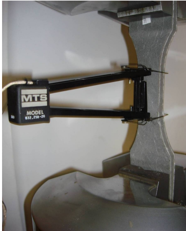
Figure 5. PU composite in-plane tensile test with extensometer.
