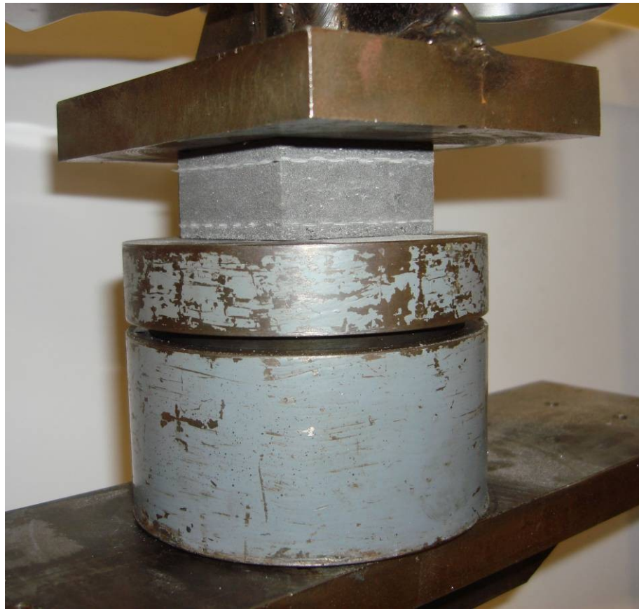
Figure 7. PU composite out-of-plane compression test.
