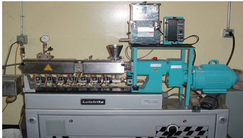
Figure 2. Leistriz Micro-18/GL-40D extruder.
