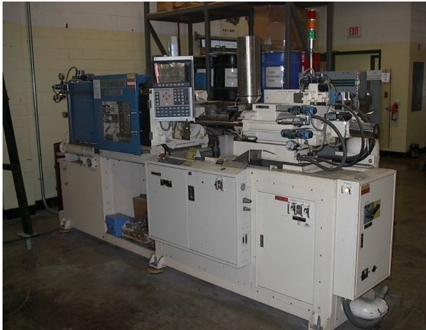
Figure 3. Technoplas, Inc. SIM 5080 injection molder.
