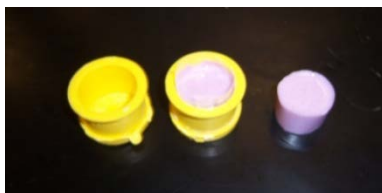
Figure 5-1. The amine-cured epoxy puck molding process: (left) the empty mold, (center) the mold with wet coating, (right) the final puck sample.
