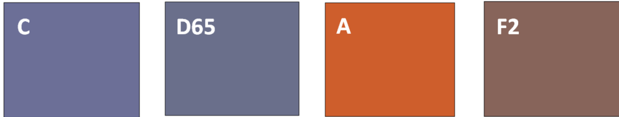
Figure 5-10. The color change program is used to simulate the visual effects of source metamerism. The violet puck is “viewed” under four different light sources (indicated by the text) using 1964 standard observer functions.
