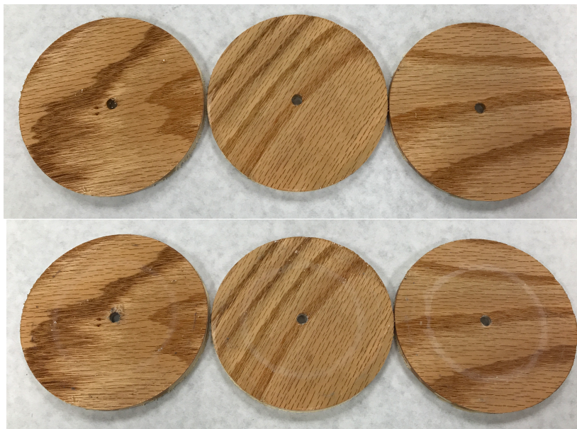
Figure 4.11. Representative coated Pine wood discs before (top) and after (bottom) abrasions.
