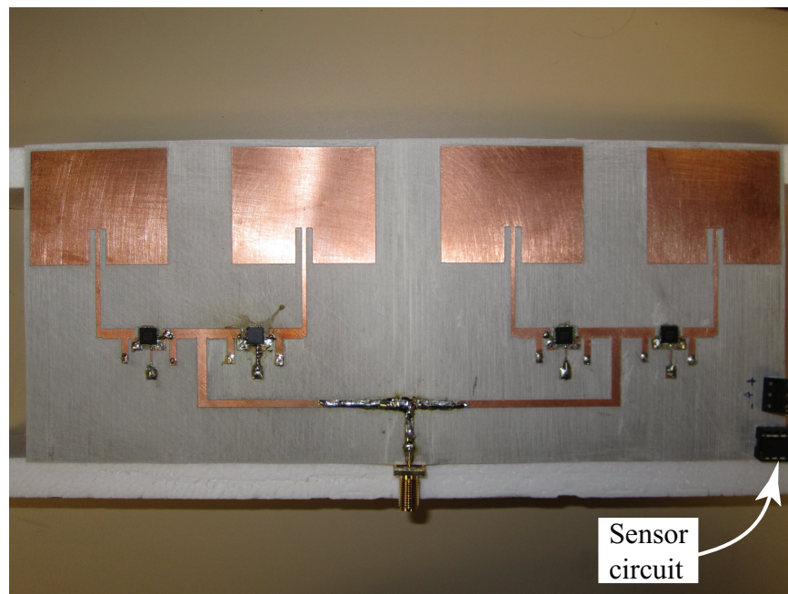
Figure 42. Picture of the manufactured 1 × 4 SELFLEX array prototype ( g = 2.0 mm, h = 35.6 mm, m = 19.8 mm, s = 11.0 mm, t = 1.3 mm, u = 33.4 mm and w = 43.6 mm).
