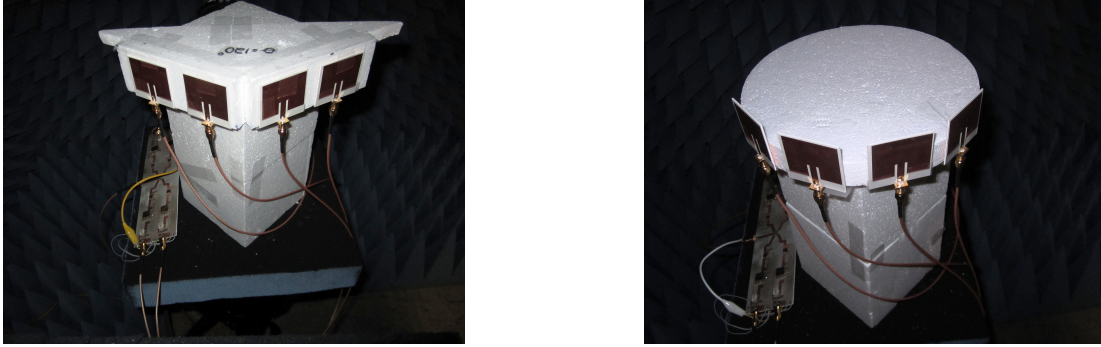
Figure 35. a) Picture of the 1 x 4 antenna test platform attached to a non-conducting wedge; b) picture of the 1 x 4 antenna test platform attached to a non-conducting cylinder.
