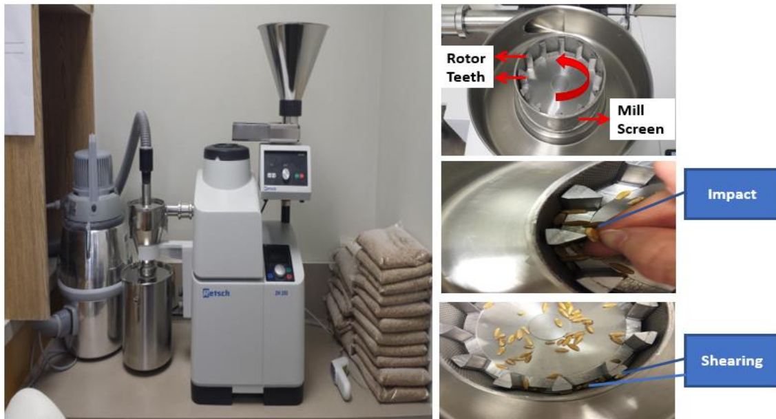
Figure 2. The ultra-centrifugal mill (left) and its grinding chamber (right).
