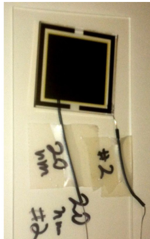
Figure 27. Device picture: One of the PVD deposited samples (absorber thickness = 20 nm) ready for characterization.
