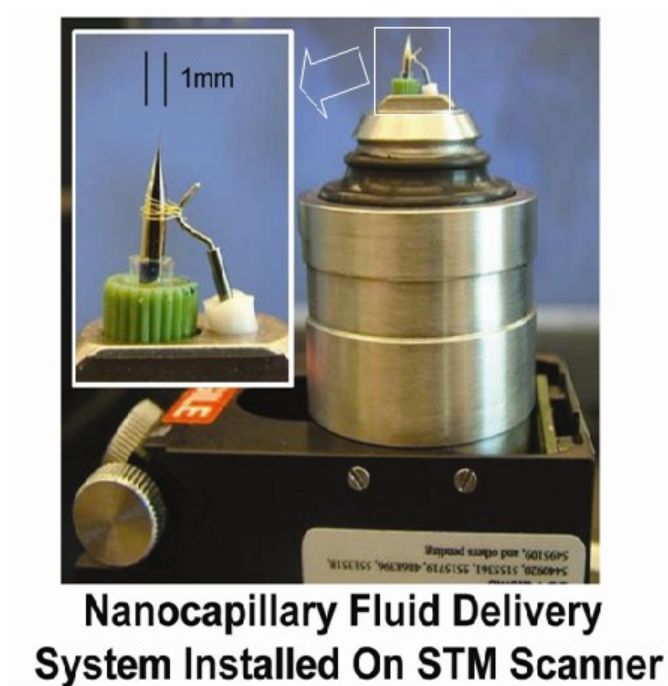
Figure 41. Hydrophobized gold-coated nano-capillary integrated in STM [18].
