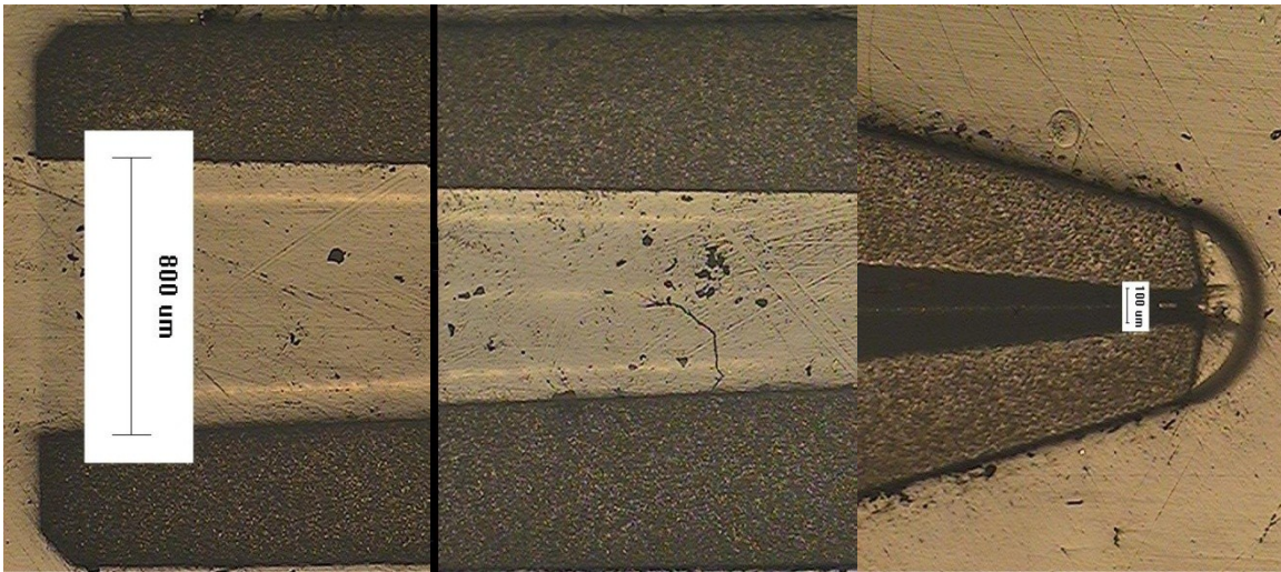
Figure 23. Ceramic 100 \mu\text{m} nozzle cross section. The geometry of a 100- \mu\text{m} nozzle can be seen above. This figure displays different cross sections of the nozzle at different magnifications. The scale can be seen on the picture. The inlet to the nozzle is on the left, while the outlet is on the right.
