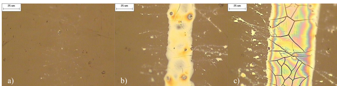
Figure 75. Printed silicon from CHS using CAB-DW on Kapton films with carrier gas flow rates of a) 5 ccm, b) 7 ccm, and c) 10 ccm.
