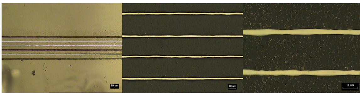
Figure 57. Lines written on double sided tape. Using flow rates of 20, 10, and 10 for the aerosol sheath and diffuser flows respectively. Line-widths appear to be approximately 3.7 \mu\text{m} .
