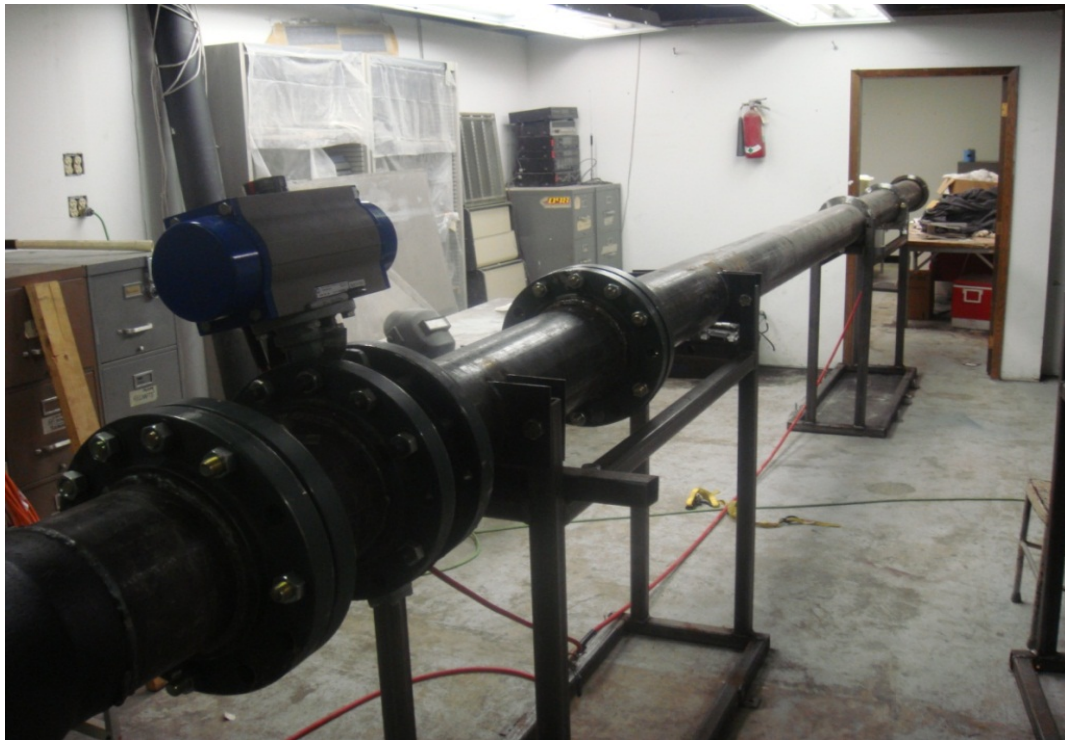
Figure 3-2: The air storage section (driver section) and the two stands holding the shock tube.
