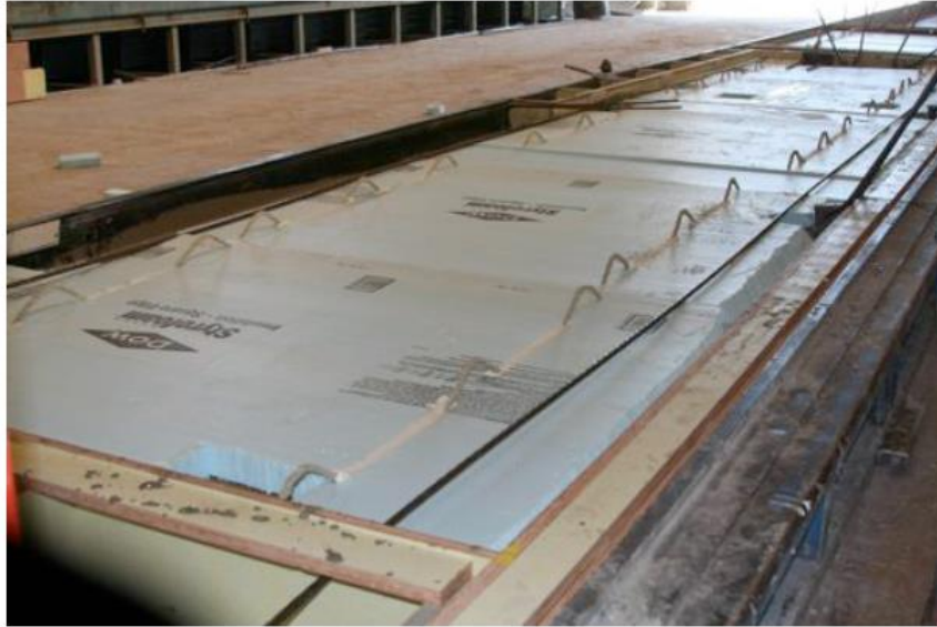
Figure 2-15: NU-tie Manufacturing Process (Morcoux et al. 2010)
