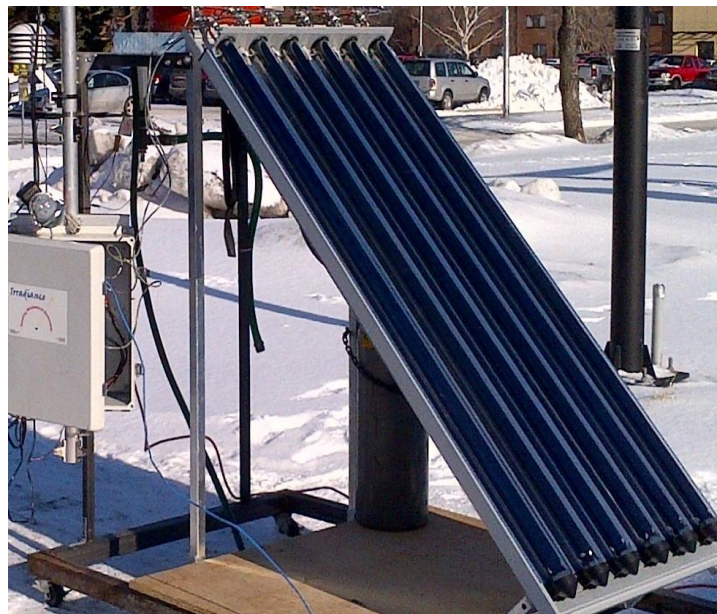
Figure 19: Evacuated tube collector
