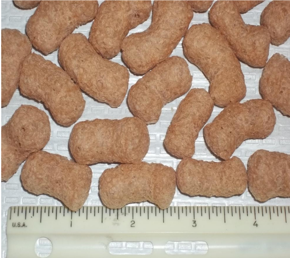
Figure 4.1. Extruded pinto bean obtained from high starch fraction. Ruler unit is in inches
