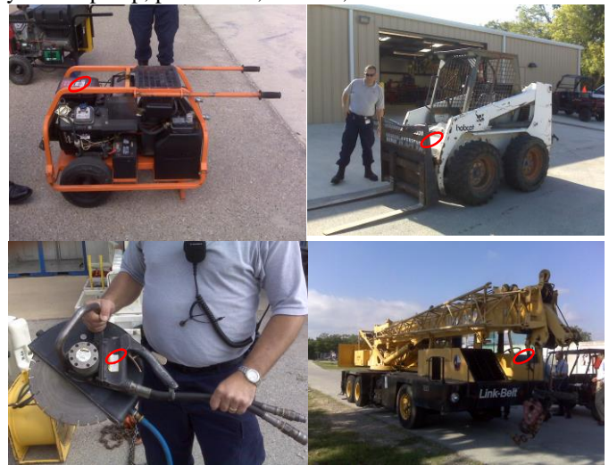
Fig. 8. Vehicles used for vibration data collection and analysis. From counter clockwise: hydraulic pump, power saw, 25 ton crane, and BobCat.
