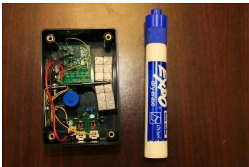
Fig. 13. EH transducer with power management and storage for Access tags.
