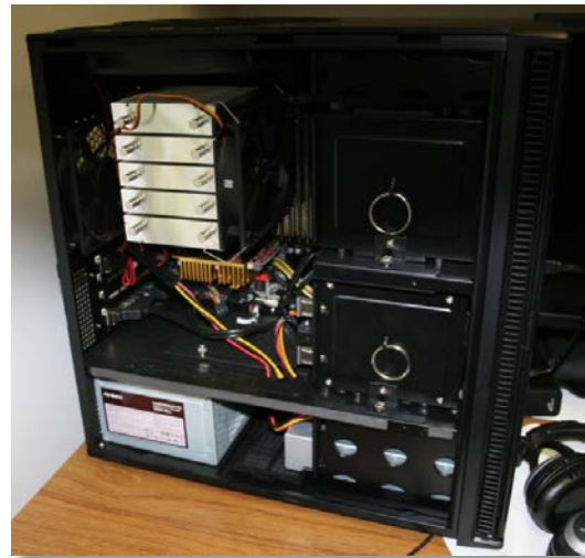
Figure B1. Computer workstation built for mitochondrial genome assembly. Computer was capable of running three mitochondrial assemblies simultaneously. General specification: Intel i7 950 (3.06GHz), 12 GB (6 x 2GB) DDR3 RAM Triple Chanel, 640GB HDD.
