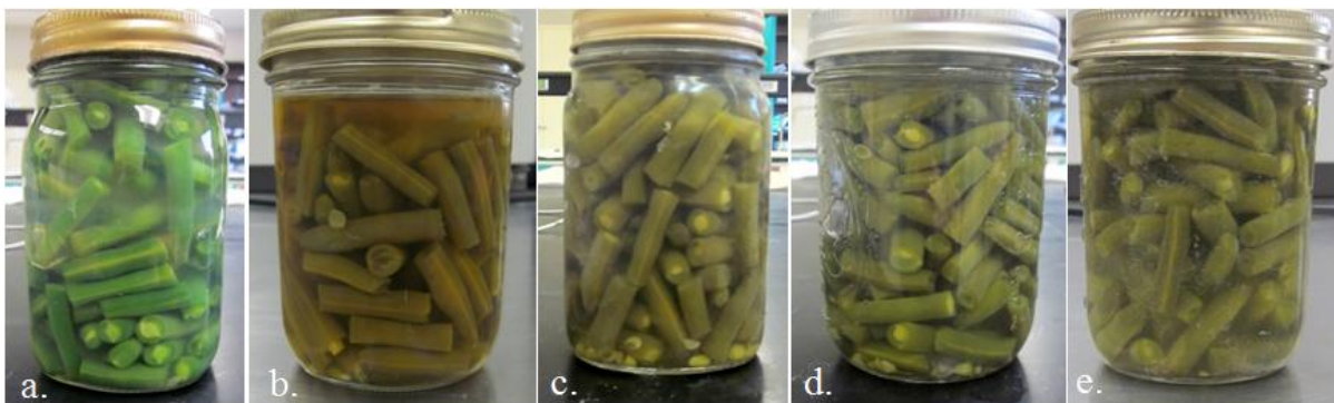
Figure 10. Green beans from various processing methods. a. control, b. pressure canning, c. boiling water bath canning, d. oven canning, e. steam canning.
