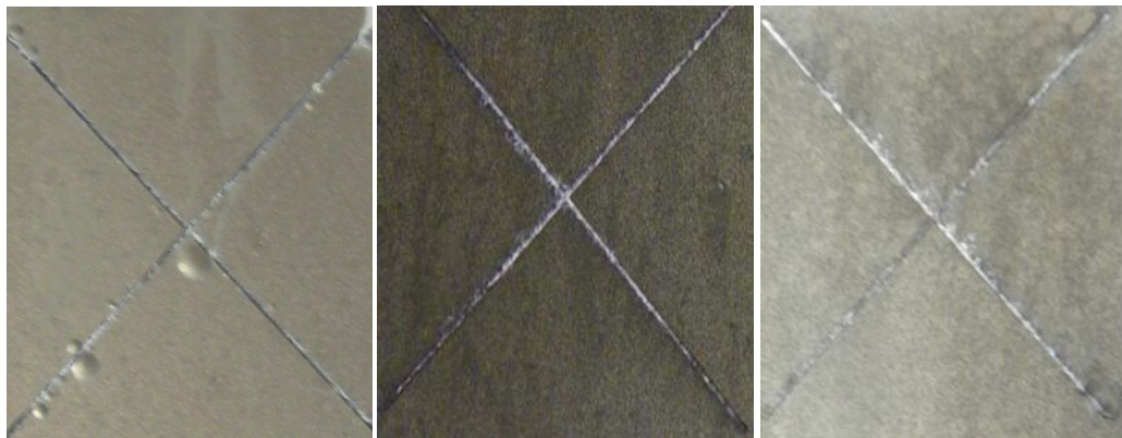
Figure 3.11: Salt spray exposure images (after 750 hours) of as received Al flake coating (left), phosphate doped PPy/Al flake coating (middle), and nitrate doped PPy/Al flake coating (right).
