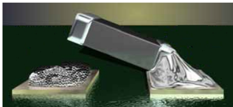
Figure 31. Tombstoned Passive Component.
