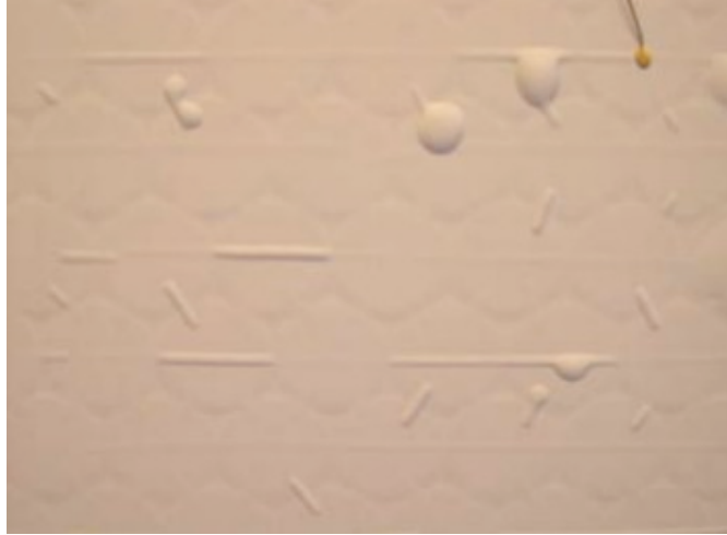
Fig. 8. Delamination of the backsheet of a PV module. 12
