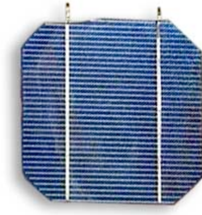
Fig. 1. Photo of an actual PV cell. The horizontal lines are the fingers and the two vertical ones are the busbars. 7
