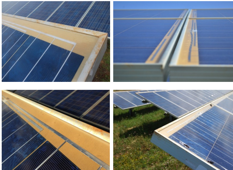
Fig. 6. Significant browning of the front encapsulant of PV modules, where most likely the polymeric encapsulant has insufficient UV stability. 12
