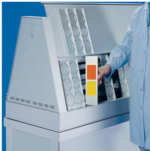
Fig. 22. QUV-SE Accelerated Weathering Tester (Q-Lab). 70
