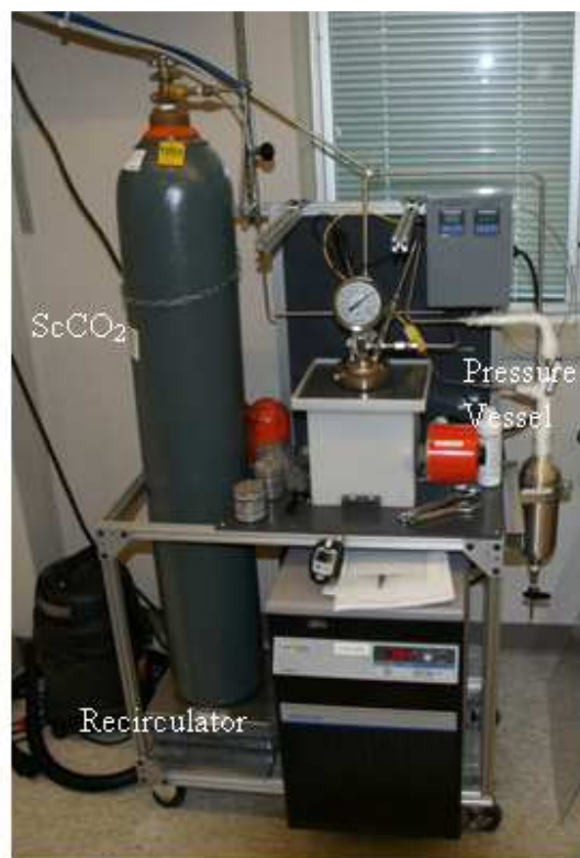
Figure 3.1. A complete reaction set-up of SCCO 2 exposure test.
