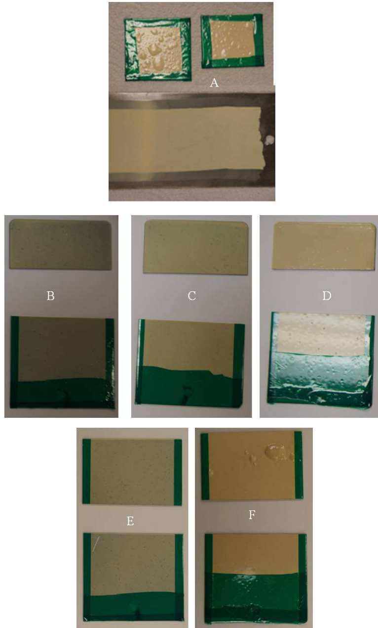
Figure 3.3. The above: coated small panels after exposure to SCCO 2 ; and the below: unexposed original panels. (A) TZ-D-107 \mu m exposed to SCCO 2 of 35 ^{\circ} C and 10.9MPa for 48 hours. (B) TZ-S-63 \mu m; (C) TZ-S-145 \mu m; and (D) TZ-S-313 \mu m exposed to SCCO 2 of 32 ^{\circ} C and 7.58MPa for 24 hours. (E) TZ-S-63 \mu m; and (F) TZ-S-313 \mu m exposed to SCCO 2 of 40 ^{\circ} C and 10.00MPa for 24 hours. (Note: the samples had to be cut to be able to fit inside the pressure vessel).
