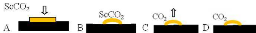
Figure 3.28. Proposed mechanism of blister formation. (A) SCCO 2 diffuses into the coatings; (B) SCCO 2 saturates the coating; (C) CO 2 diffuses out of the coatings when pressure is reduced to atmospheric pressure; and (D) Remaining CO 2 changes into gaseous phase and causes blistering with extreme volume increase.
