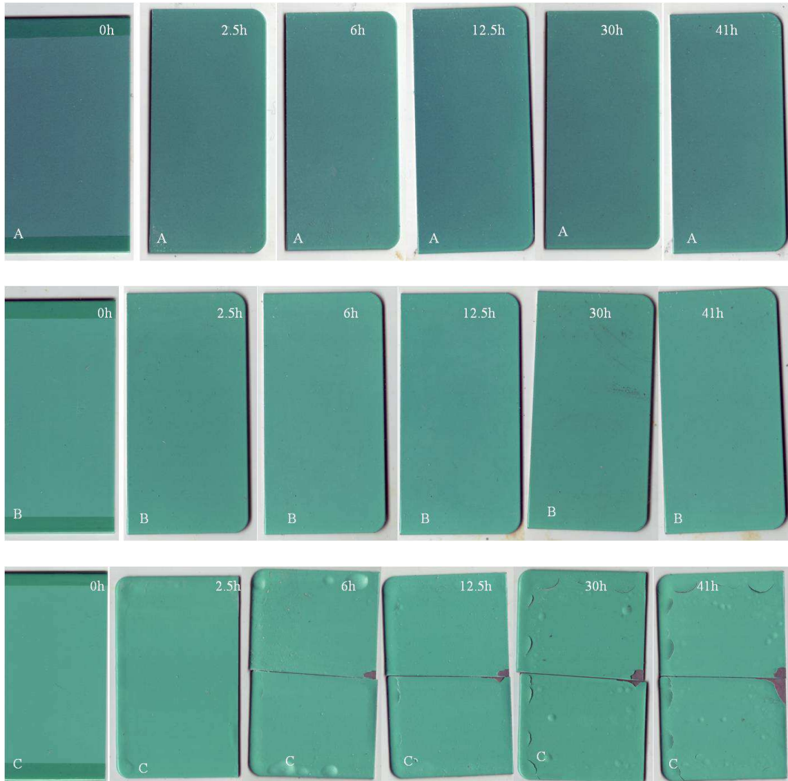
Figure 3.13. Coated panels with different exposure time to SCCO 2 of 32°C and 7.58MPa for 24 hours. A: S323-S-35µm; B: S323-S-65µm; and C: S323-S-172µm.
