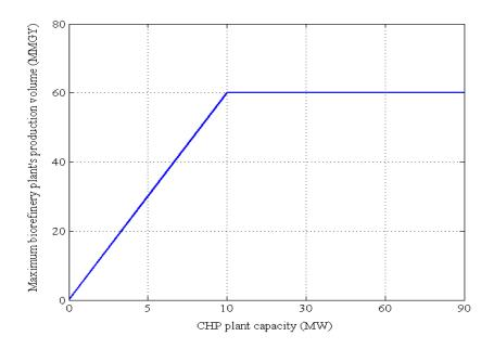
Figure 19. Impact of the CHP plant capacity on the biorefinery plant
