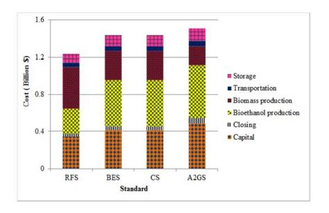
Figure 33. Total bioethanol supply chain cost under different standards
