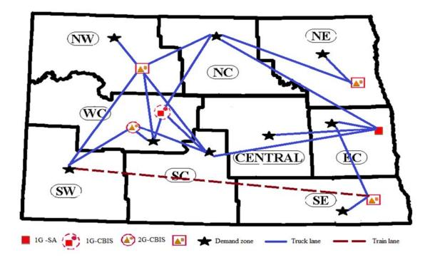
Figure 72. Network topology of bioethanol plant to demand zone in ISHGBSC under RFS
