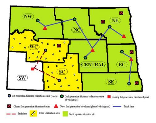
Figure 40. Network topology of biomass supply sites to bioethanol plants in HGBSC at state 'B'
