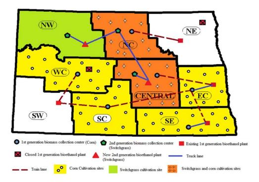
Figure 39. Network topology of biomass supply sites to bioethanol plants in HGBSC at state 'A'
