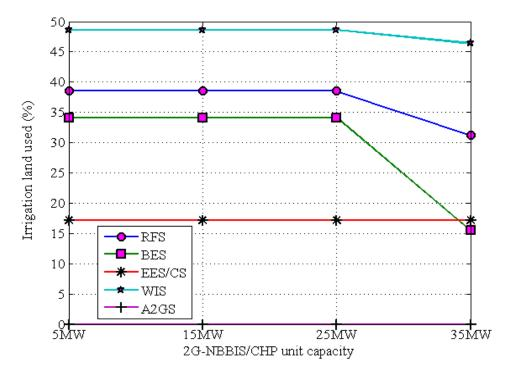
Figure 81. Irrigation land used by ISHGBSC when CHP unit capacity of 2G-NBBIS is increased
