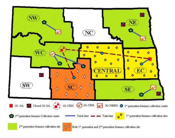
Figure 70. Network topology of biomass supply to bioethanol plant in ISHGBSC under RFS
