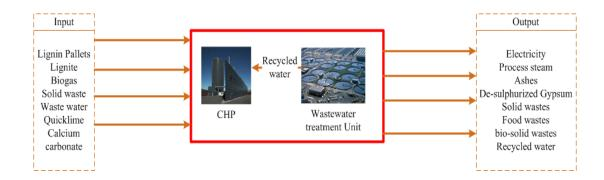
Figure 8. Input and output products of the CHP plant
