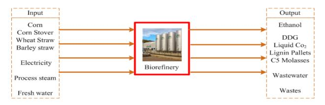
Figure 7. Input and output products of the biorefinery plant
