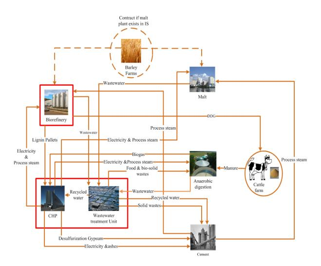
**Figure 6.** Candidate plants and their potential SLs \*Biorefinery Plant and CHP Plant – anchor tenants (Highlighted by red boxes) \*Dash lines indicate potential combined contract by biorefinery plant and malt plant with barley farms
