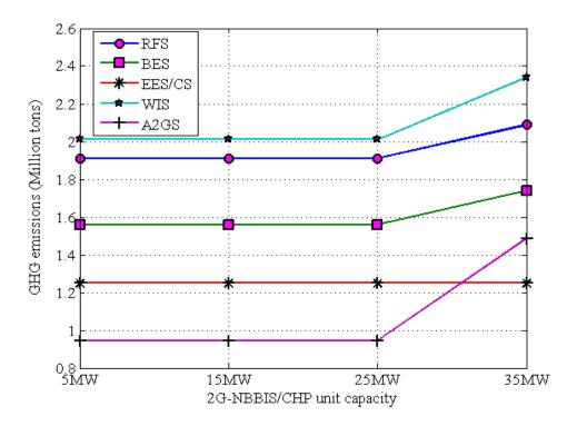
Figure 80. GHG emissions of ISHGBSC when the CHP unit capacity of 2G-NBBIS is increased
