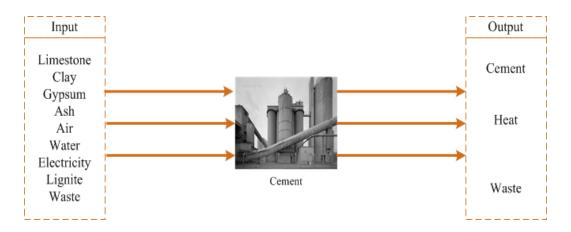
Figure 10. Input and output products of the cement plant
