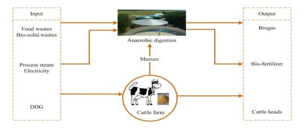
Figure 9. Input and output products for the AD plant
