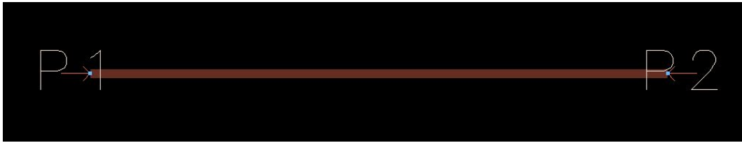
Figure 5.12. ADS layout for the test microstrip transmission line with a characteristic impedance of 50 \Omega .
