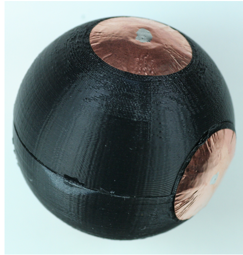
(b) Alternate view of the fully assembled antenna.
