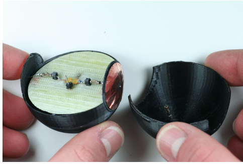
(a) Partially assembled antenna from the side.
