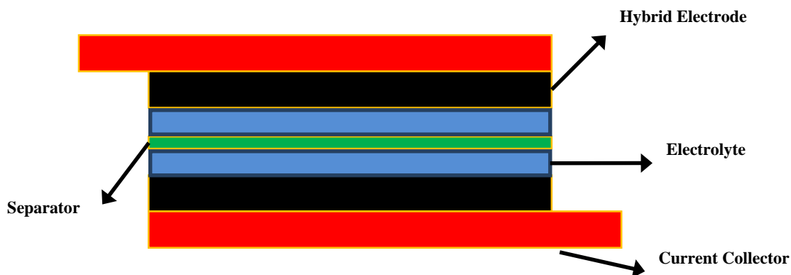
Figure 3.1. Schematic of a solid-state supercapacitor.
