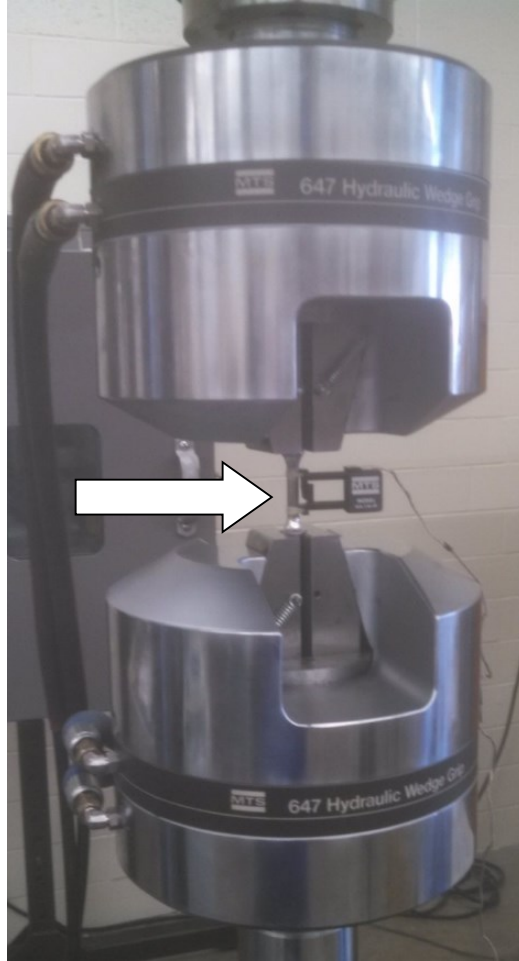
Figure 5.1. MTS load frame with a LCF specimen installed.
