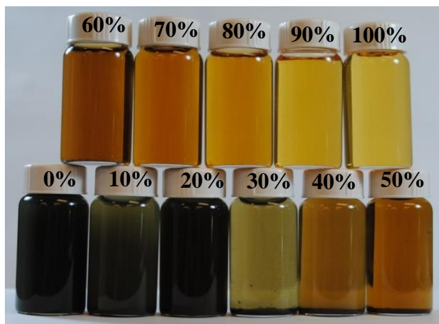
Figure 3.6. Image of vials after 7 days of the reaction at various methanol concentrations. (Methanol concentration on the vials in volume %)
