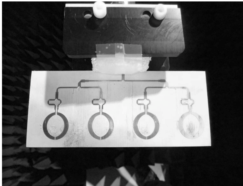
Fig. 52. Close-up view of split-ring antenna array mounting system.
