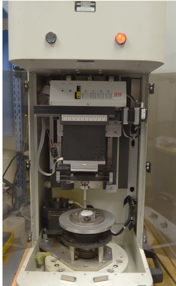
Figure 2.2: CETR-UMT-2 pin-on-disc tribometer set-up.
