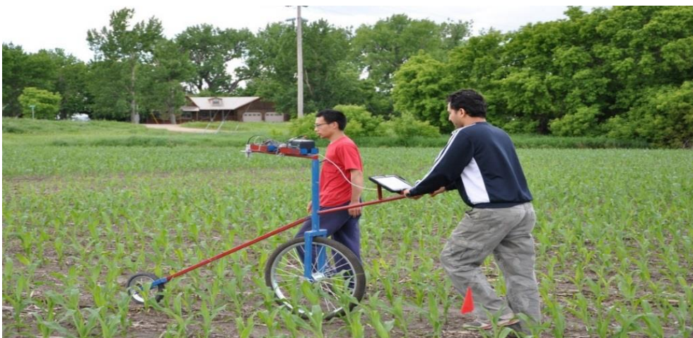
Fig. 1. Method of collecting data from SenixVIEW height sensor mounted on bicycle while connected with Dell Latitude 10ST2e.
