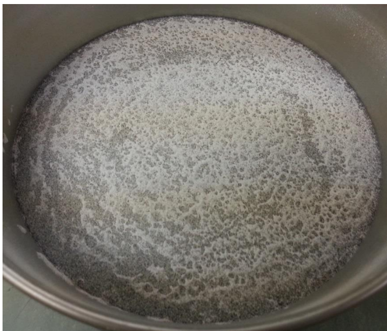
Figure 28. Fine flour on top blocked by the layer on the bottom.
