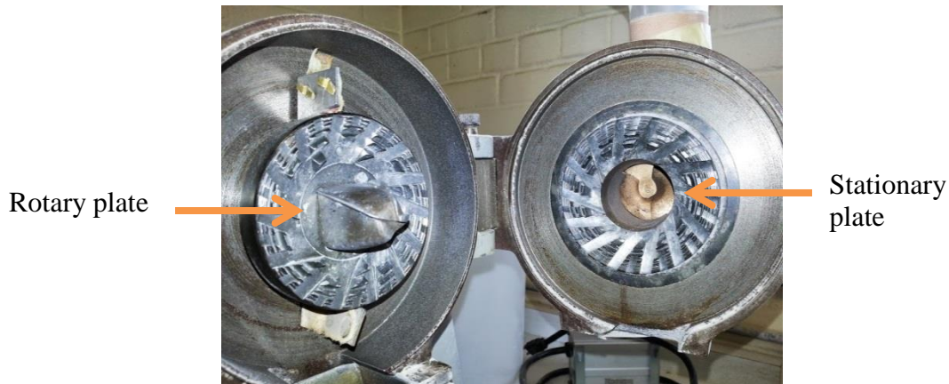
Figure 3. Open burr mill and its plates.
