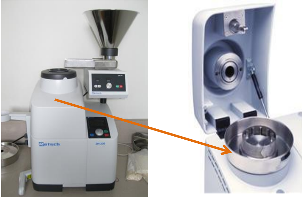
Figure 2. Centrifugal mill (left) and the rotor with the screen (right).
