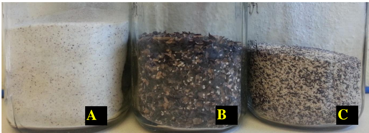
Figure 31. Cotyledon flour (A), seed coat fraction (B), and by-product (C) after burr mill/roller milling system.
