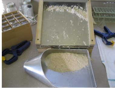
Figure 10. Residue left behind by the formulation 100% whole wheat flour hydrated at 15% on the stainless steel surface after running the angle of slide test.
