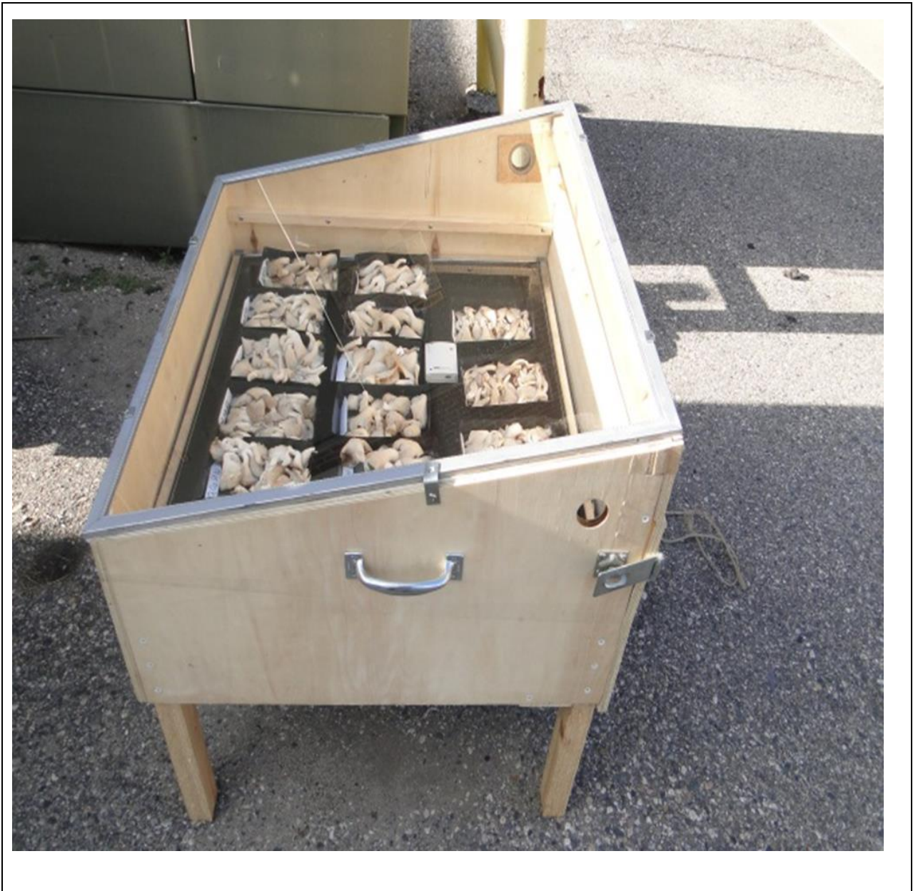
Figure A15. Solar drier #1 used for oyster mushroom drying, summer 2011.
