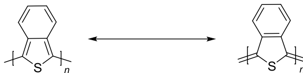
Figure 1.7. Non-degenerate resonance forms of isothianaphthene (PITN)
