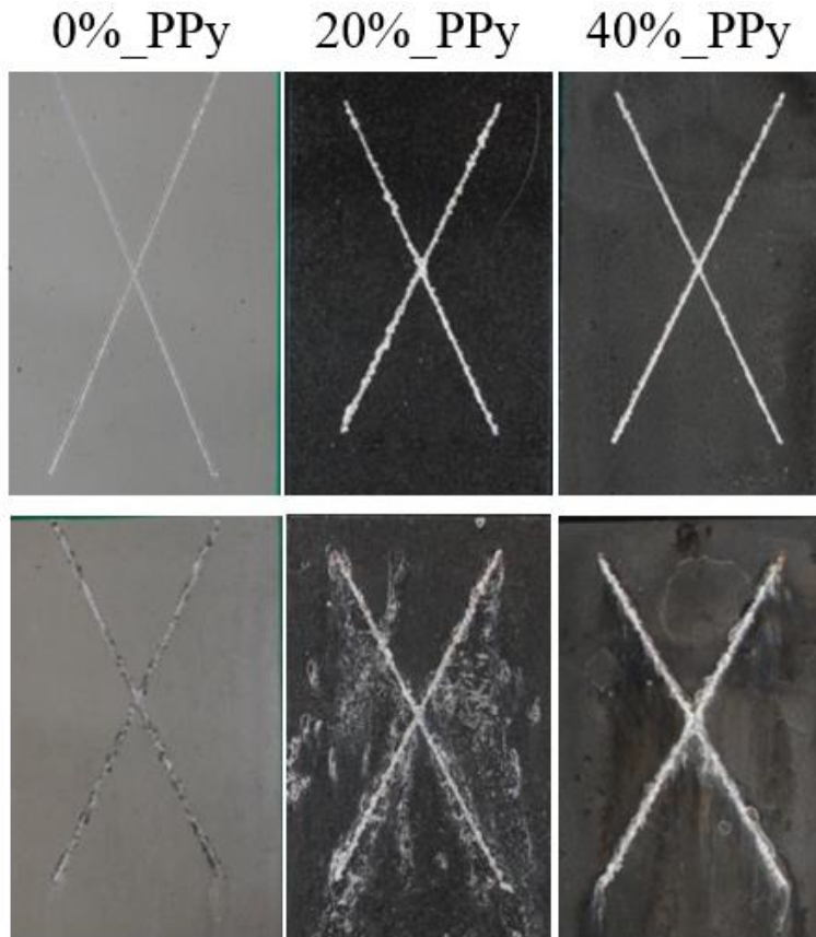
Figure 3.9: Optical photographs of ASTM B117 salt spray results. Top – prior to exposure, Bottom – after 168 hours exposure.
