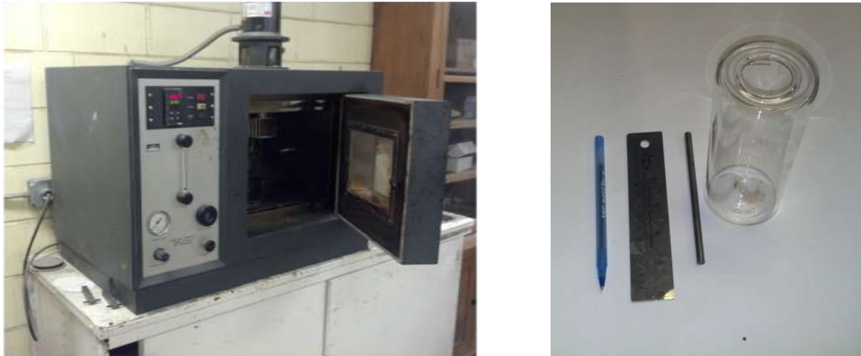
Figure 3-2: RTFO and the bottle and rode configuration
