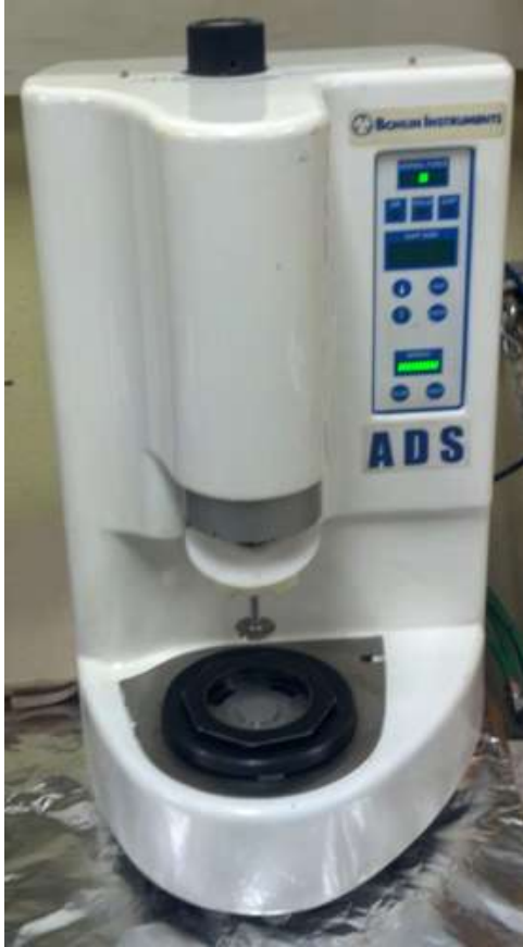
Figure 3-1: Dynamic shear rheometer and plate geometry
