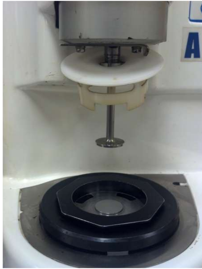
Figure 3-1: Dynamic shear rheometer and plate geometry
