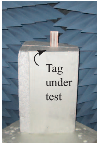
Figure 22. Prototype antenna design I being measured in the anechoic chamber.
